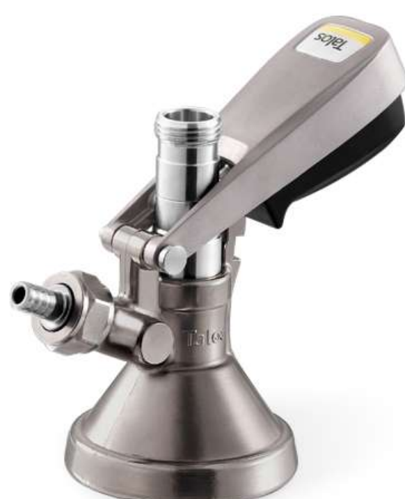
PART NO.: 1023601 Tin-nickel Brass Body, 304 S.S Probe Without Pressure Relief Valve
